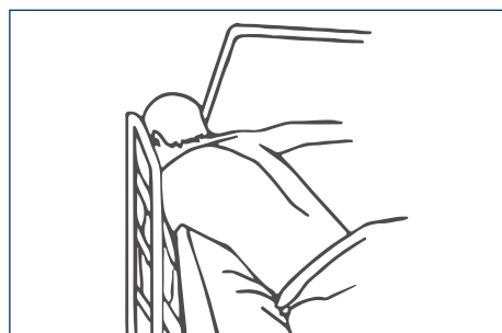
Zone 6: Between the End of the Rail and the Side Edge of the Head or Footboard
