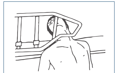
Zone 4: Under the Rail, at the Ends of the Rail
