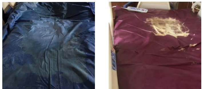
Figure 1: Top Cover Damage
